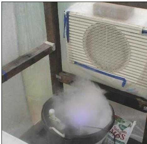
**Photo 9: Evaporative cooler and humidifier.**
